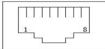
Figure 3.7 Ethernet RJ45 pin definition
